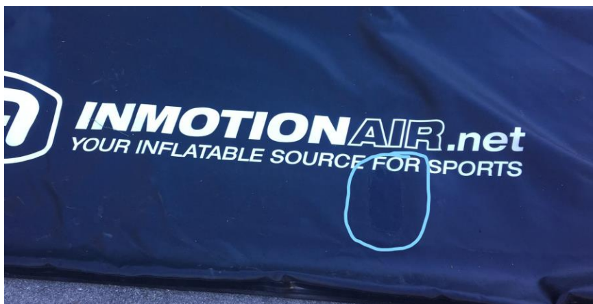
Exterior patch used in 2-layer sandwich patch shown in the circled area above in photo.
